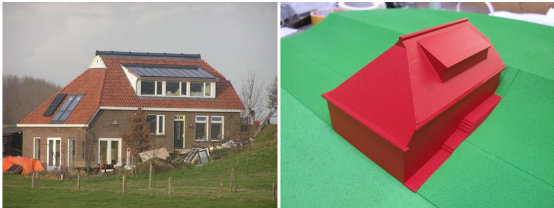
Test house for full scale experiments (left), and corresponding wind tunnel model.
